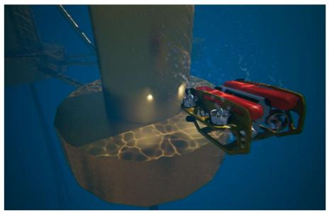
Artist's impression of an AUV inspecting the floater of a floating wind turbine. The presence of turbulence in the current flowing around the structure, its constant motion, and the presence of waves will act to make the manoeuvring of the AUV much more challenging than in commonly encountered situations. This poses a need for advanced control systems that we are aiming to develop.
