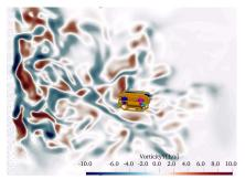
AUV manoeuvring in a turbulent flow generated inside a viscous computational fluid dynamic (CFD) simulation. Our access to such advanced computational tools allows us to simulate the hydrodynamics of AUV motion with much higher accuracy than using more traditional approaches. This additional insight allows us to better design and evaluate control systems before they will be tested on the actual vehicles.
